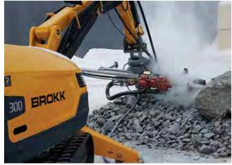
The MMB326 hydraulic drifter rock drill attachment.
