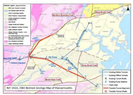
The quality of rock encountered along the City Tunnel is noted by Tierney as being excellent for tunneling. Just 5 m (16 ft) of the 7.7-km (4.78-mile) tunnel required structural steel support with the remaining approximately 7.7 km (4.7 miles) of tunnel mined with no need for temporary supports. The bedrock through which the City Tunnel extends was considered unusually good as compared to that encountered along other tunnels previously mined through similar geology in the greater Boston area.
